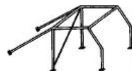
Dimensions 38mm dia x 2.5mm thick or 40mm dia x 2.0 thick. Note: These figures represent minimums. In selecting the steel, attention must be paid to obtaining good elongation properties and adequate weldability. The tubing must be bent by a cold working process and the centreline bend radius must be at least three times the tube diameter. If the tubing is ovalised during bending, the ratio of minor to major diameter must be 0.9 or greater.
